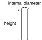
When small test-tubes are provided, it is expected that these are approximately 150 mm in height.
